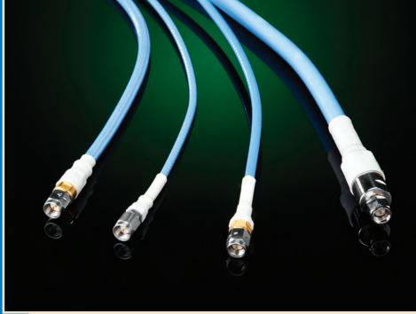
Phase Track® cable assemblies are designed for applications demanding minimal phase change over temperature. All Phase Track cables use proprietary  $TF4^{TM}$  dielectric that does not have the abrupt shift in the phase that occurs with solid or tape wrapped PTFE based products under normal room ambient temperature conditions.
