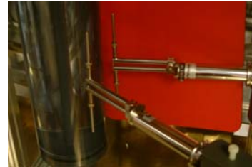
Example of simple two-dipole diversity antenna located 2 cm from a cylinder filled with tissue-equivalent liquid. Results are given below.
