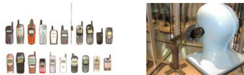
The 20 measured phones (left) and example of hand phantom used in other measurements. (right).
