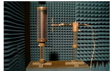
Bluetest RC800 reverberation chamber and setup for antenna measurements. The field is stirred by 2 mechanical stirrers, a platform stirrer, polarization stirring and 25 MHz frequency stirring.
